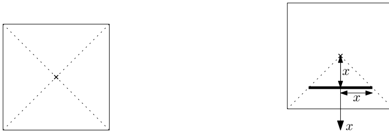
(a) We divide the cube diagonally into quarters. (b) We divide a quarter of the plate into thin strips of width dx . If their distance is x from the center of the wafer, their length is 2x .
