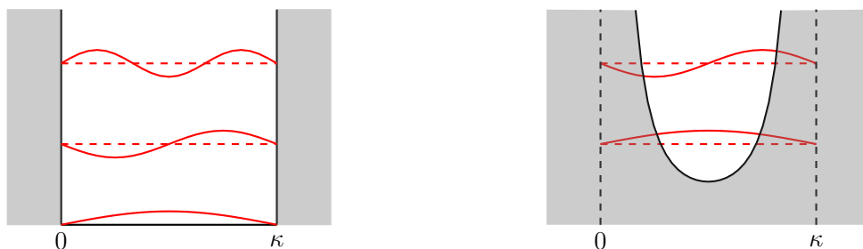
Figure IV: Low lying eigenstates of the square potential well (left) as well as the first member of eq. 2.23 (right). The first excited state of the square well corresponds to the ground state of the second potential.
