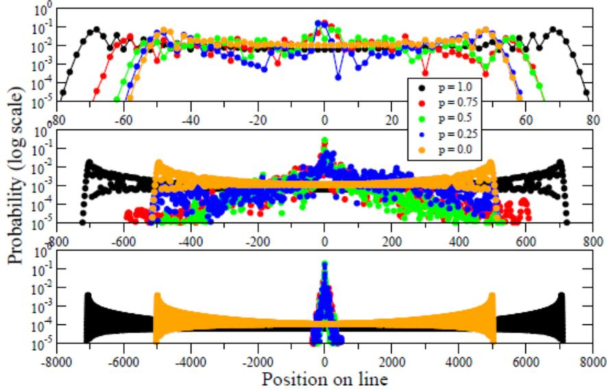
Figure 3.1: Quantum walk with tunnelling ( $\eta = 0.25$ ) with various setting: 100 (top), 1000 (middle) and 10000 (bottom) steps with percolation probability  $p = 1$  (black), 0.75 (red), 0.5 (green), 0.25 (blue) and 0 (orange). Only even positions are displayed, since probability at odd positions is zero in even time steps. [4].
