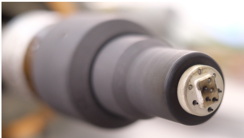
Figure 18: Visual inspection of the probe after the CC15.04 campaign showed damaged edges of the boron nitride bulk.
