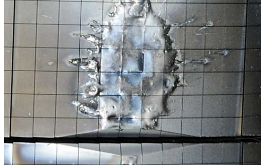
Figure 1.1: Re-deposited molten beryllium appears on tiles inside the JET vessel after experiments focused on RE generation and effects.[1]
