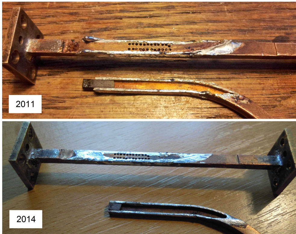
Figure 3.13: Directional coupler - desoldered
