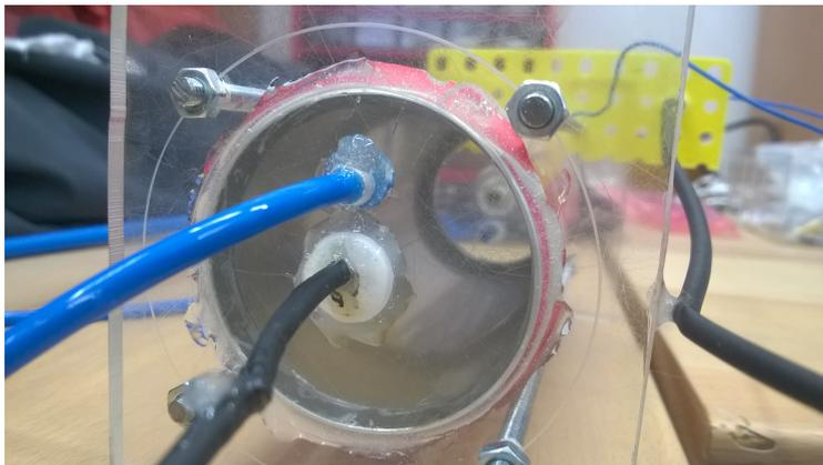
Fig. 2.2: Gas proportional can, end cap detail.
