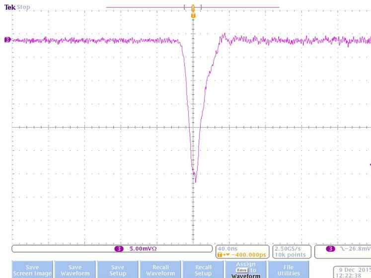
Fig. 3.2: Measured pulse from the photomultiplier.
