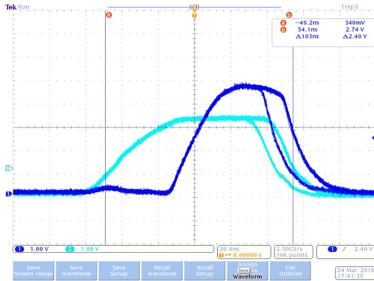
Fig. 3.4: Blue: signal before the IGBT. Cyan: signal before the coincidence unit.
