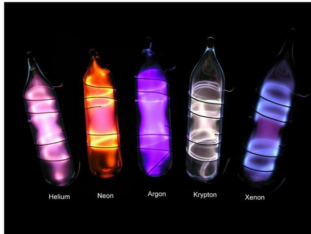
Fig. 2.2: Discharge in high purity (99.999%) helium, neon, argon, krypton and xenon in vacuum. [4]
