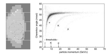
• Cherenkov rings detected by system of multichannel photomultipliers
