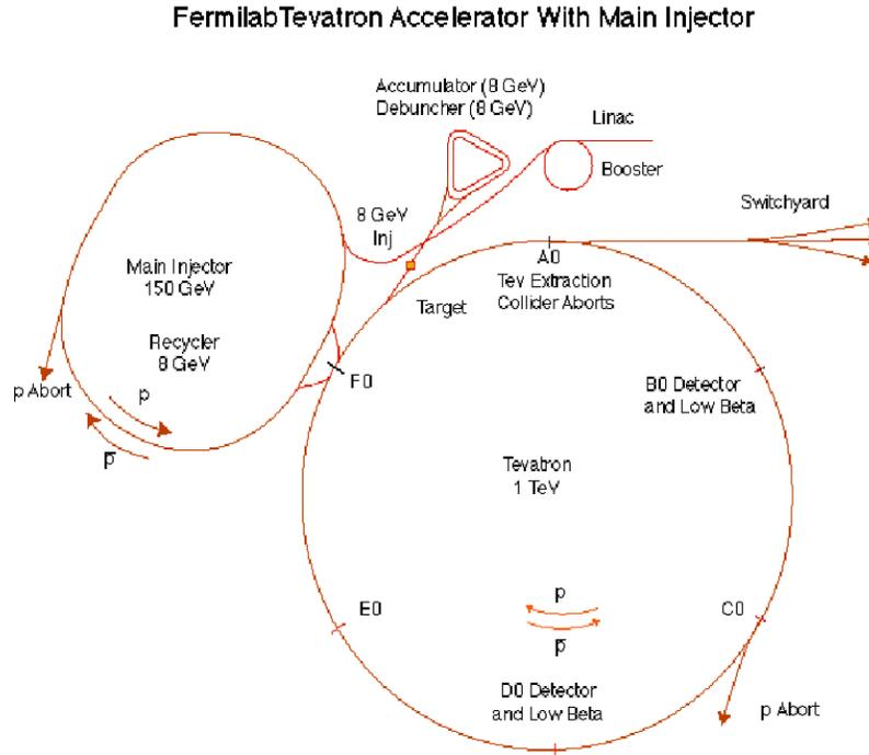
Figure 2.1: The scheme of Tevatron accelerator. It is described in the text. The picture was taken from [21].
