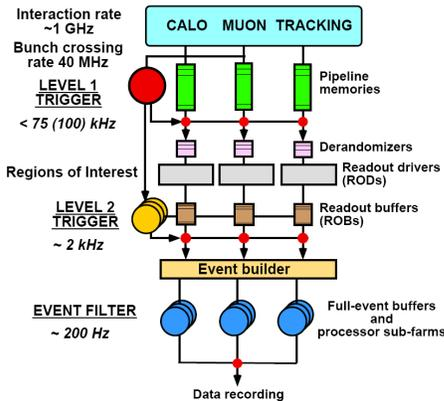
Figure 2.8: The scheme of ATLAS trigger. The picture was taken from [27]
