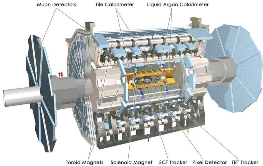
Figure 2.6: The ATLAS detector. The picture was taken from [28].
