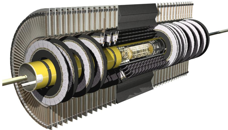
Figure 2.7: The Inner Detector. The visible core is pixel detector. Around it, there is SCT and on the outskirts, there is TRT. The picture was taken from [28].
