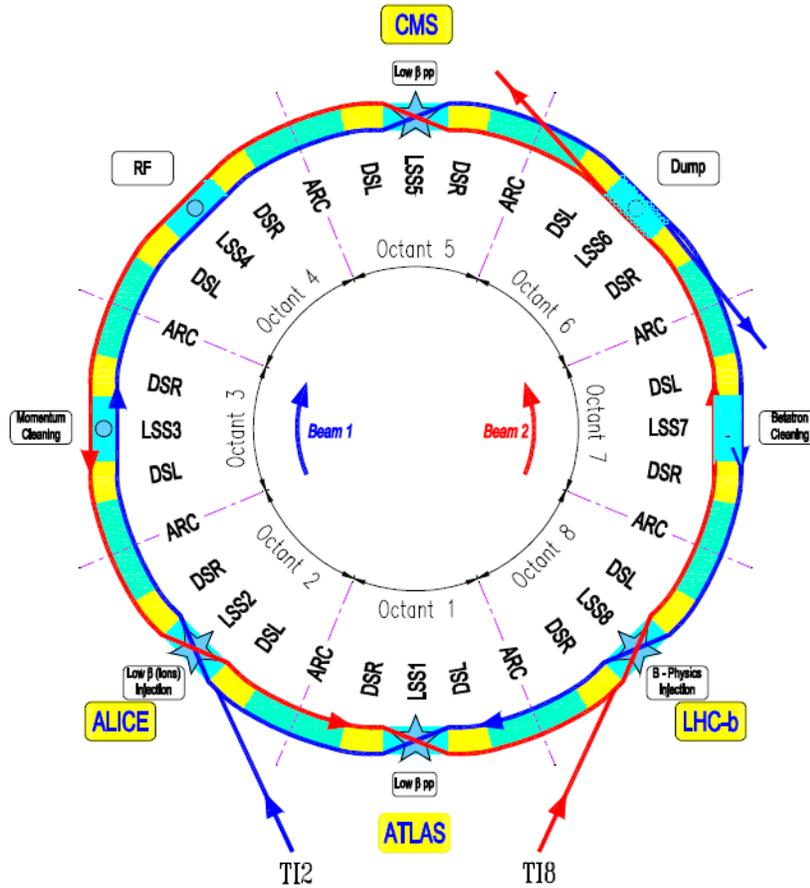
Figure 2.5: The scheme of LHC. It shows the location of experiments and other Insertion regions. The picture was taken from [30].
