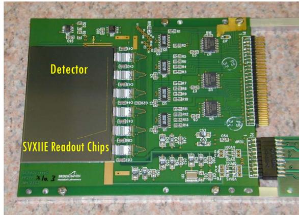
Fig. 3.11: A photo of the plane. Detector and SVXII readout chips are highlighted. Taken from Ref. [62].
