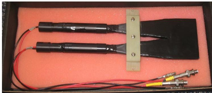
Fig. 3.12: A photo of the trigger counter of single detector package. Taken from Ref. [65].
