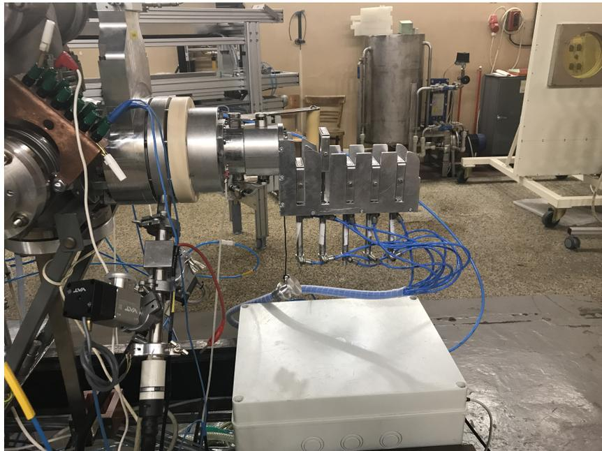
Figure 3.8: Photo of the degrader unit with aluminum plates behind the beamline exit window. During the irradiation, we used the 0.55 mm thick aluminum plate to make the beam profile wider. The initial energy of the proton beam is about 35 MeV. After passing through the degrader plate and air it reduces to  $\sim 30$  MeV at the sample position.
