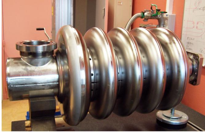
Figure 3.2: Superconducting radiofrequency cavity operating at 700 MHz. Taken from Ref. [76].
