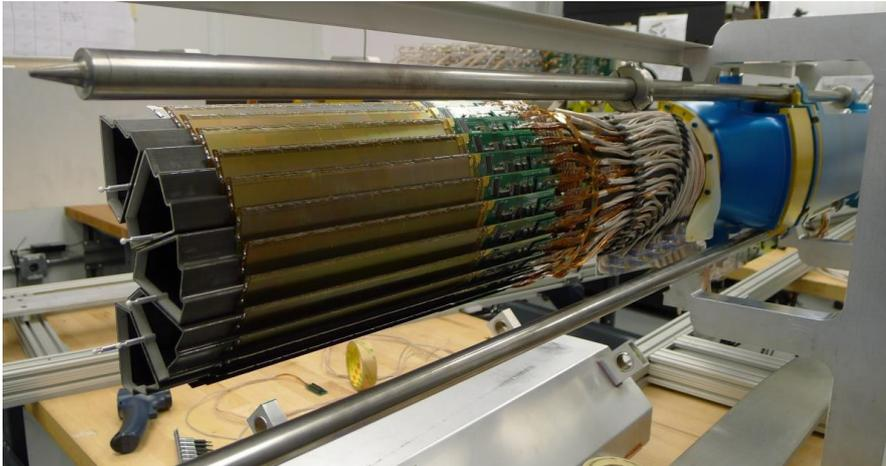
Figure 3.8: Structure of the Pixel detector. The sectors are grey and are carrying ladders with detectors, the readout cables are on the far side. Taken from Ref. [51].
