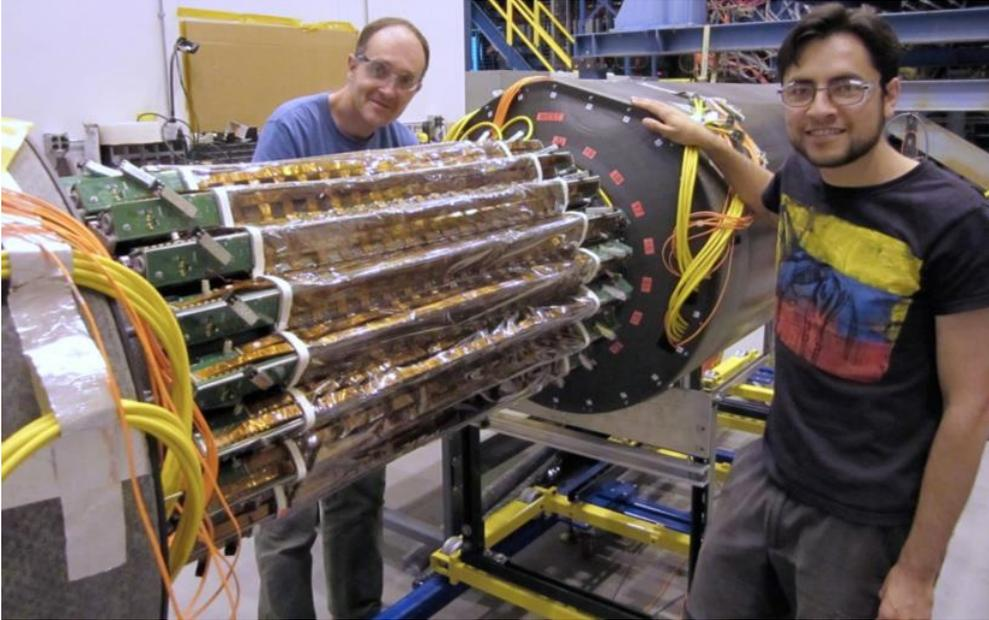
Figure 3.6: The SSD team during detector installation. Taken from Ref. [51].
