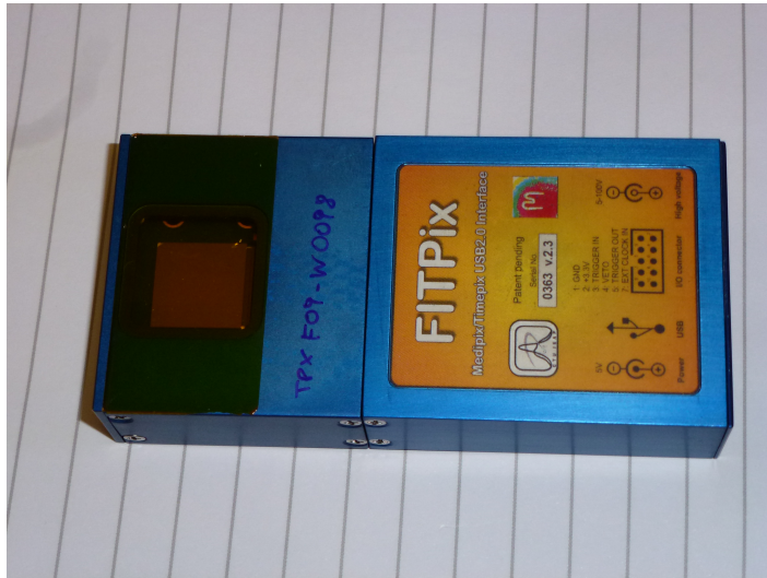
Figure 2.9: Timepix chip used in our measurements. [27]
