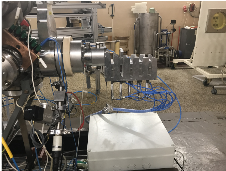
Figure 3.8: Photo of degrader plates system behind the beam pipe exit window, in our experiment only one plate was used.
