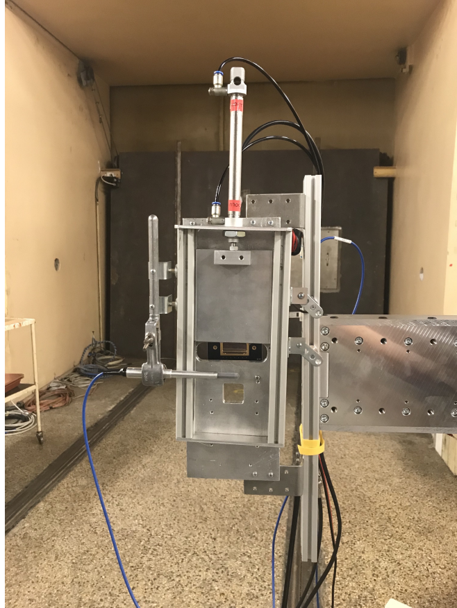
Figure 3.9: Photo of the frame with the ionization chamber, beam stop plate and the ALPIDE chip, all placed on the arm of the movable stage. The relative position of ALPIDE and the ionization chamber is fixed, the beam stop plate covers the chip during the beam profile scanning.
