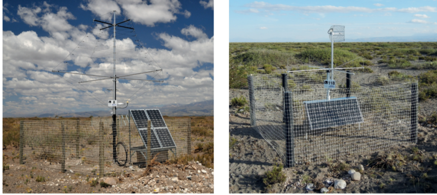
Figure 2.5: Antennas used in the Observatory for the detection of the electromagnetic component of a shower. Left: A logarithmic periodic dipole antenna. Right: A butterfly antenna [25].
