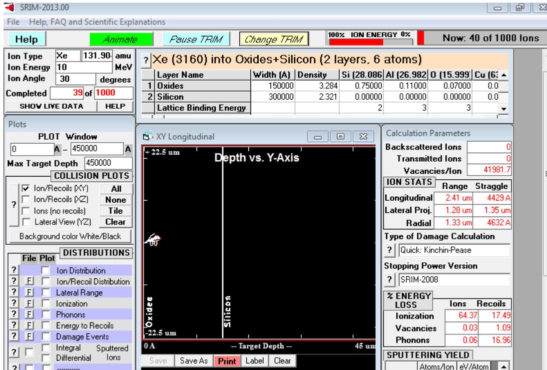
Fig. 4.3. The process of simulation in SRIM software.
