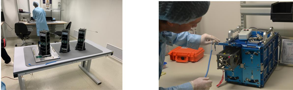
Fig. 6.2. Left: Three CubeSats ready for the launch. The first from right is containing the Czech module. Right: The deployer that is responsible for the ejection of the CubeSat once it is on the sun synchronous orbit.
