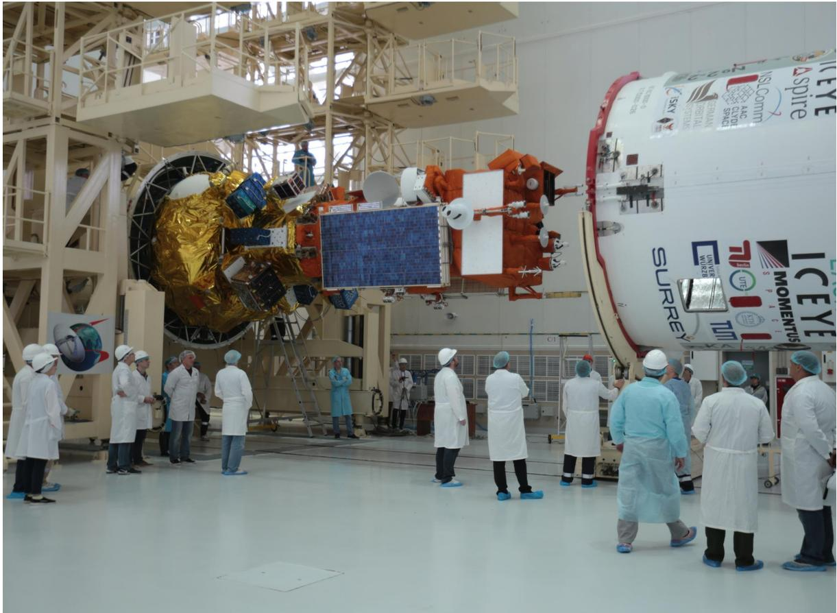
Fig. 6.3. The detail of the mission arrangement. The dominating part equipped with the solar panel is weather satellite Meteor M2-2. On the left, deployers with CubeSats are mounted.
