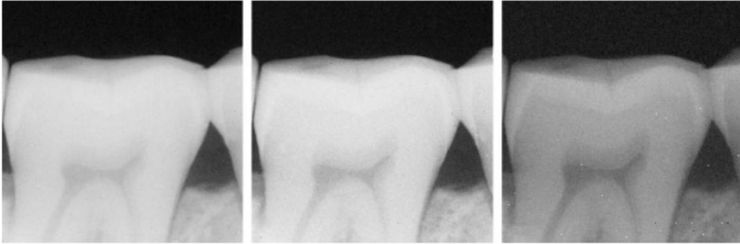
Fig. III.15: Images of a tooth (molar) taken by Medipix2 detector using a conventional X-ray tube. Energy window dependent image quality. Window energy are set like 4-8 keV, 26-30 keV and 45-49 keV from left to right. Taken from [13].
