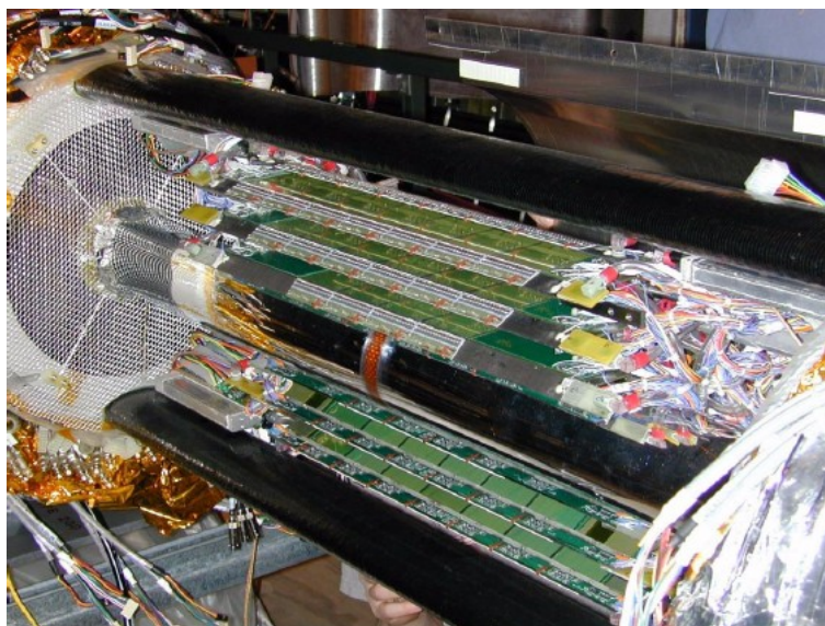
Fig 8.5 SVT in middle of construction
