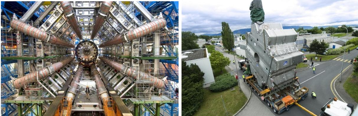
Figure 2.6: Left: The eight toroidal magnets can be seen on the huge ATLAS detector with the calorimeter [21]. Right: ATLAS magnet toroid end-cap [22].
