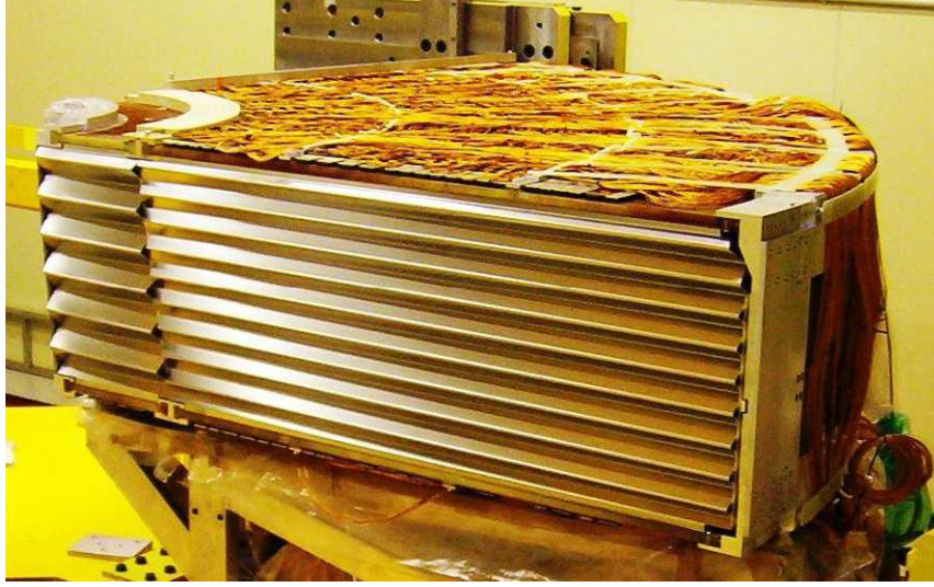
Figure 3.13: Photograph showing a side view of an electromagnetic end-cap LAr module
