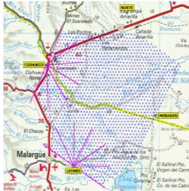
Figure 5.3: The final scheme of all surface detectors (blue points) used at PAO in Argentina. The yellow labels represent the places, where are the fluorescence telescopes placed.
