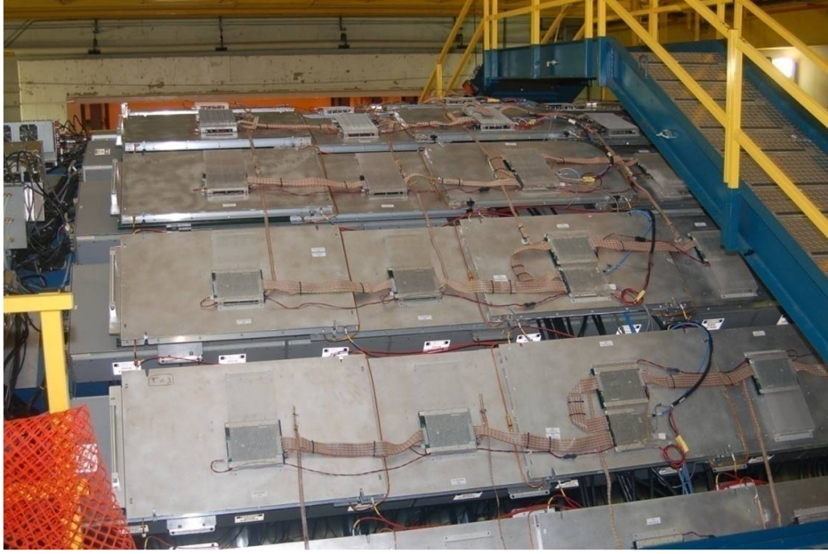
Figure 2.6: View of MTD detector and its position on the outside of the STAR detector. Each row consists of 5 MTD modules (not all 5 are visible in the picture), at the bottom of the detector some rows consist of less modules due to space constraints.
