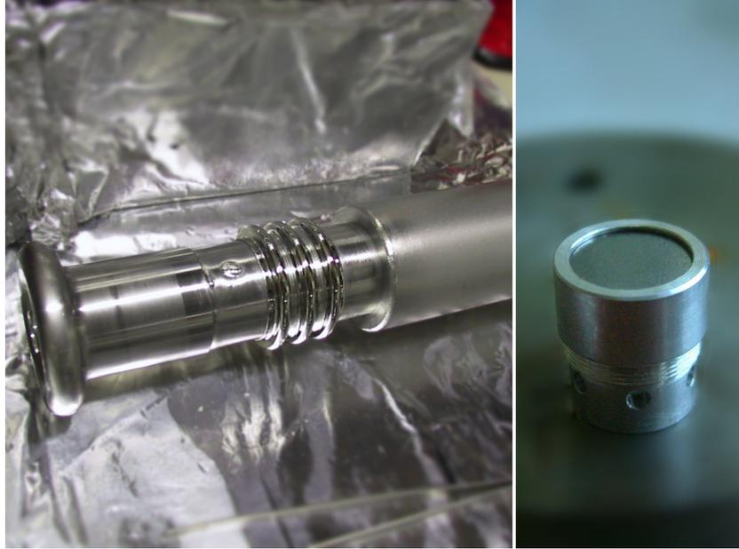
**Figure 4.2** The former holder of quenched condensed tritium modified to house a  $^{83}\text{Rb}/^{83\text{m}}\text{Kr}$  source. A detail picture of the  $^{83}\text{Rb}/^{83\text{m}}\text{Kr}$  source on the right.
