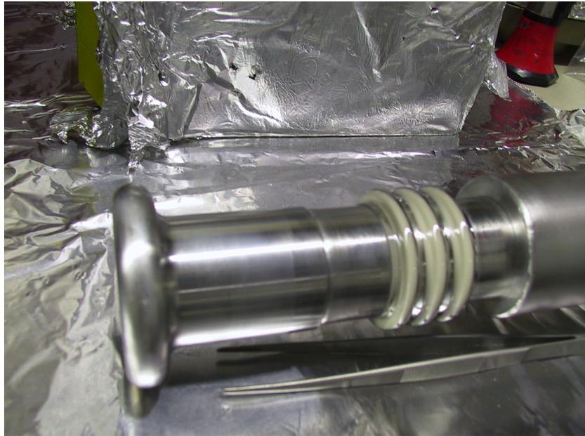
**Figure 4.42** An insulator to separate the cup with the  $^{241}\text{Am}/\text{Co}$  source and the guiding tube. It was partially coated with steel during the Ar etching of the Co foil. The setup should be improved to avoid such coating.
