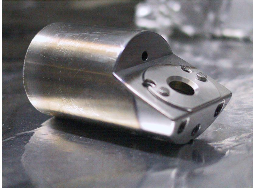
**Figure 4.27** A holder of an electron source for the tilted geometry to cut down background.
