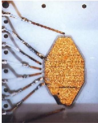
Figure 3.8.: START diamond strip detector.
