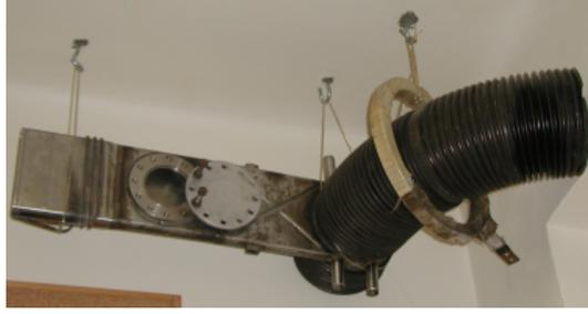
Figure 4.2: A sample from liner replaced in 1984, encircled by coil of toroidal magnetic field generation.
