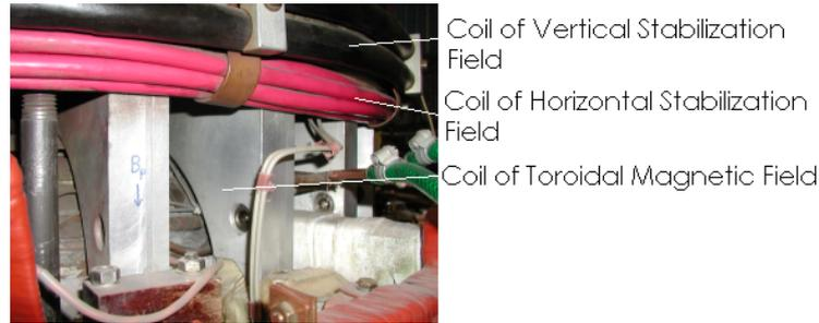
Figure 4.6: Coils of toroidal and poloidal magnetic field generation.
