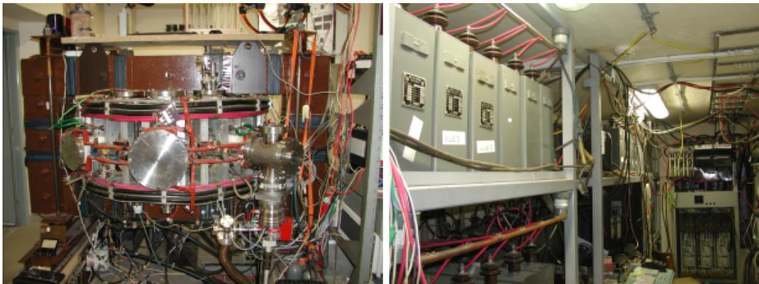
Figure 4.1: Present status of tokamak GOLEM. Tokamak itself is on the left panel while room for containment of energizing systems is on the right panel.
