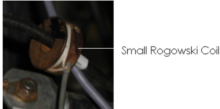
Figure 4.10: Small Rogowski coil used for measurement of currents flowing through conductors.
