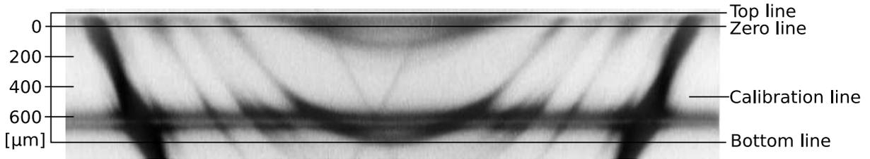
Figure A.2: Raw spectral data as should be loaded in VJS Analyser, with the horizontal lines marked on the right.
