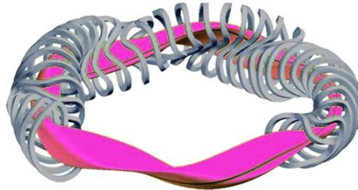
Figure 1.3: Model of stellarator coils; reprinted from [7].
